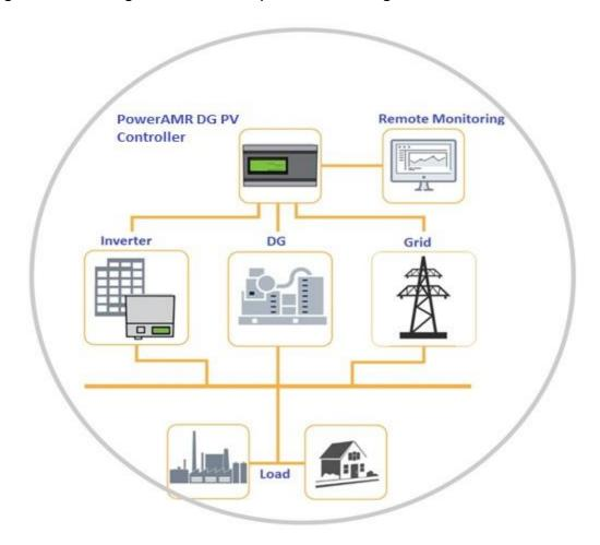
When we get off status from the grid and ON status from DG or DG'S, the DG sync controller will throttle power of each Inverter as per building load. It also divides user load between DG and solar smartly in such way that DG will run at minimum load and solar cater maximum part of user load. This will result in the minimum fuel consumption of DG along with reverse power protection and solar optimized.
