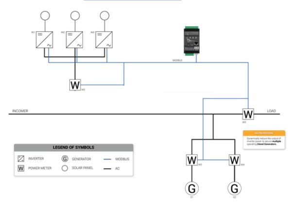
• In case of DG Synchronization, meter shall be installed at DG panel.
